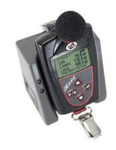
**Sound Level Meter** – Used for acoustic (sound that travels through air) measurements. It is commonly a hand-held instrument with a microphone.
